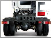
▲ Bigger axle capacity with reinforced frame chassis (12mm).
